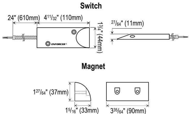
**Note:** On wood surfaces, the magnet shall be installed at least 1/4" from the switch housing to comply with UL 681 installation requirements.
